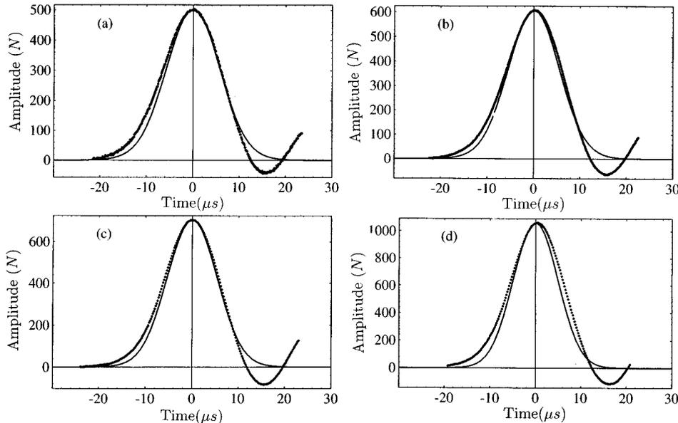
FIG. 7. Same as Fig. 6, with the same notations, but for greater values of  $\psi_m/\psi_\infty$ . The respective characteristics of each pulse are (a)  $F_m = 503$  N,  $V = 1060$  m/s,  $\psi_m/\psi_\infty = 10.4$ ; (b)  $F_m = 608$  N,  $V = 1086$  m/s,  $\psi_m/\psi_\infty = 11.8$ ; (c)  $F_m = 705$  N,  $V = 1106$  m/s,  $\psi_m/\psi_\infty = 13.0$ ; and (d)  $F_m = 1060$  N,  $V = 1168$  m/s,  $\psi_m/\psi_\infty = 17.0$ .
