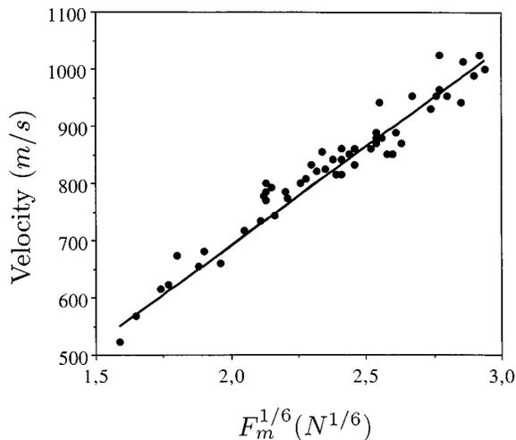
FIG. 16. Graph of the wave velocity (in m/s) as a function of  $F_m^{1/6}$  (in  $N^{1/6}$ ), where  $F_m$  is the maximum amplitude of the wave, when no static force is applied on the chain; the relation is clearly linear, which simply states that the Hertz interaction between adjacent beads is responsible for wave propagation.
