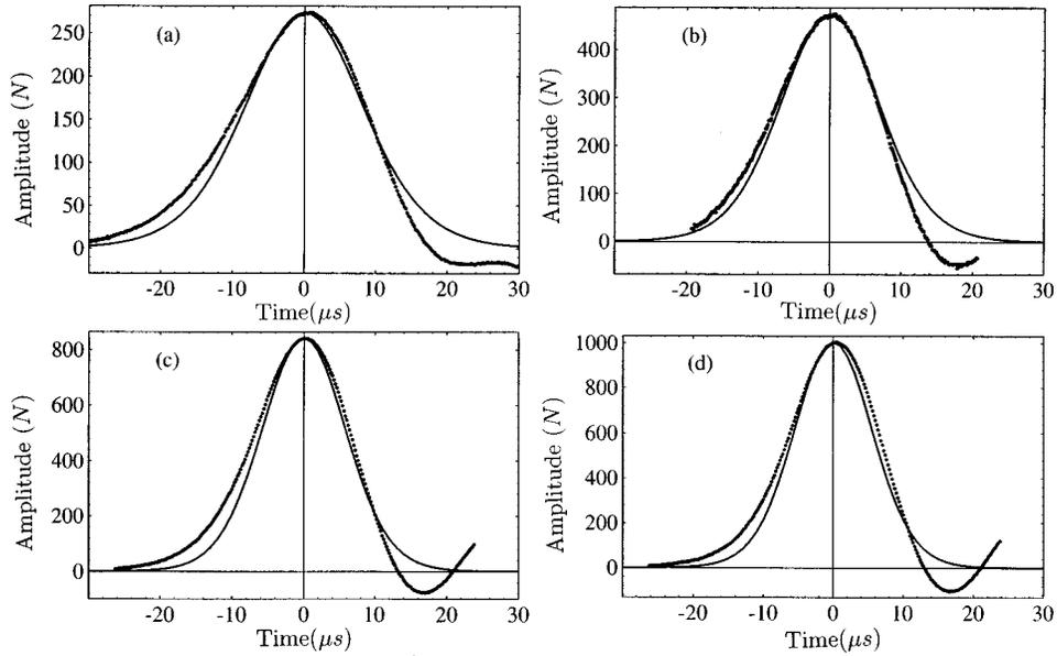
FIG. 8. Same as Fig. 6, with the same notations, but for a static force of 167 N. The respective characteristics of each pulse are (a)  $F_m = 274$  N,  $V = 1131$  m/s,  $\psi_m/\psi_\infty = 2.5$ ; (b)  $F_m = 474$  N,  $V = 1178$  m/s,  $\psi_m/\psi_\infty = 3.3$ ; (c)  $F_m = 842$  N,  $V = 1239$  m/s,  $\psi_m/\psi_\infty = 4.7$ ; and (d)  $F_m = 1005$  N,  $V = 1260$  m/s,  $\psi_m/\psi_\infty = 5.2$ .
