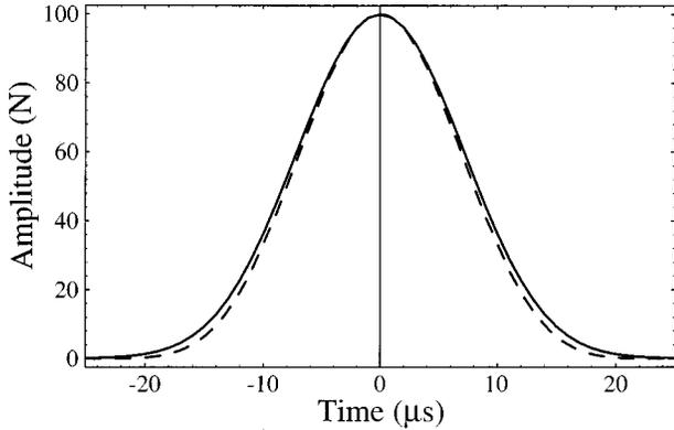
FIG. 2. Evolution of the force (in N) as a function of time (in  $\mu\text{s}$ ) for a maximum amplitude of 100 N and, respectively, a static force of 1 N (solid line) [the wave profile is determined by Eq. (23)] and no static force (dashed line) [the wave profile is determined by Eq. (28)]. The similarity of the two curves is striking; the chosen value of 1 N roughly corresponds to the available resolution on the static force (see Sec. III A).
