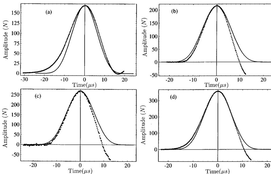
FIG. 14. Same as Fig. 13, but for waves of greater amplitudes. The velocities and amplitudes of the pulses are, respectively, (a)  $V=811$  m/s,  $F_m=168.5$  N; (b)  $V=845$  m/s,  $F_m=216.2$  N; (c)  $V=877$  m/s,  $F_m=269.7$  N; and (d)  $V=919$  m/s,  $F_m=356.4$  N. The negative part of the force signal at the back of the pulses in (b)–(d) is the signature of the sensor resonance. The agreement with the theory is very satisfactory and much better than for the pulses of Fig. 13.
