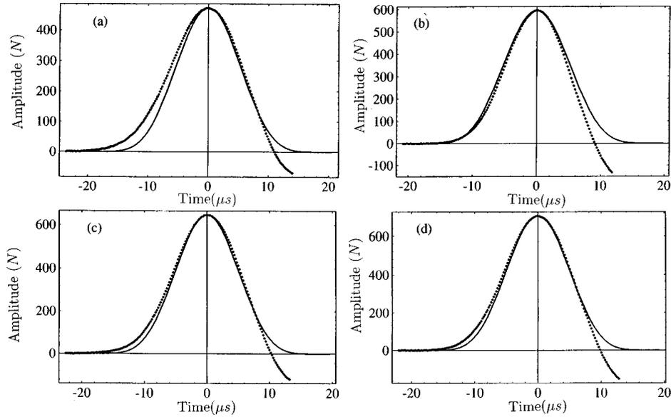
FIG. 15. Same as Figs. 13 and 14, but for waves of greater amplitudes. The velocities and amplitudes of the pulses are, respectively, (a)  $V=963$  m/s,  $F_m=473.1$  N; (b)  $V=1000$  m/s,  $F_m=594.0$  N; (c)  $V=1014$  m/s,  $F_m=646.1$  N; and (d)  $V=1029$  m/s,  $F_m=704.6$  N. The negative part of the force signal at the back of the pulse is the signature of the sensor resonance. As in Fig. 14, the agreement with the theory is very good.
