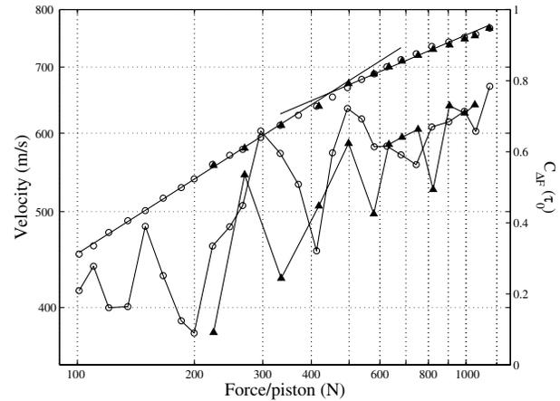
FIG. 3. Left ordinate: plot, in log-log scale, of the velocity versus the applied force, in steel beads, during compression ( $\circ$ ) and decompression ( $\blacktriangle$ ) of the same lattice. Right ordinate: plot, in log-linear scale, of the correlation  $C_{\Delta F}(\tau_0)$  [cf. Equation (3)] (same symbols, joined by a solid line).
